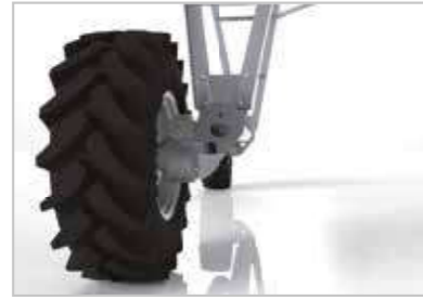
High level of rigidity thanks to the wide angle brackets
