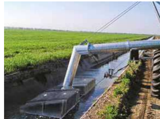
Individual solution: floating suction line
